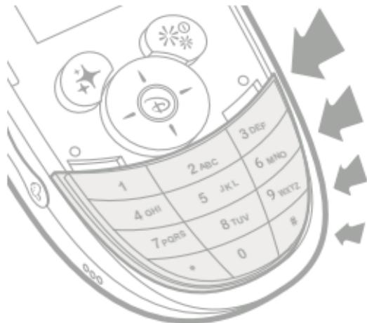
2 As you continue around the perimeter of the keypad, ensure that its four side tabs locate correctly. If any key sticks up then its stud may not be correctly seated.
