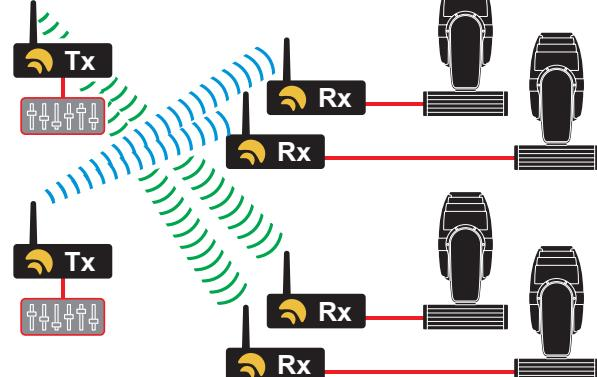
W-DMX™ is unique in its use of certain advanced radio techniques which are more often found in mobile phone and military communications. Rather than using fixed frequency channels, W-DMX™ uses adaptive frequency hopping technology (as well as TDMA and GFSK techniques) to continually check for interference and to rapidly move operation over to clear radio channels. The frequency hops occur one thousand times every second to ensure smooth, efficient and robust operation.
